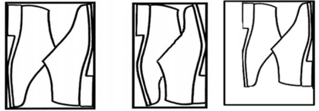
F11. The shoe box size must be of a suitable size for the footwear (left figure), ensuring there is no excessive movement of the footwear (right figure) within the box; alternatively, the shoe box is too small (figure in the middle), which could damage the product.
