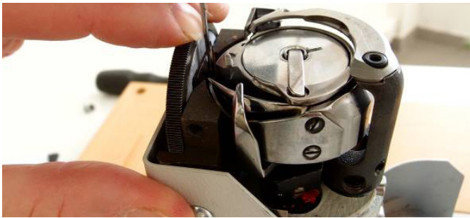
F.64 Frequent mistake: The protection plate is not properly adjusted and the hook touches the needle.
