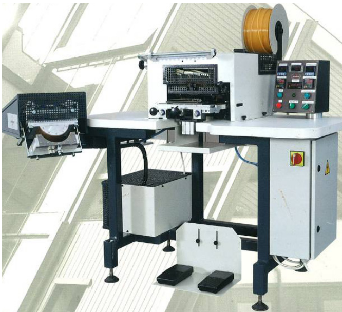
F.51 Example of a sustainable way of toe-puff application with hotmelt adhesive
