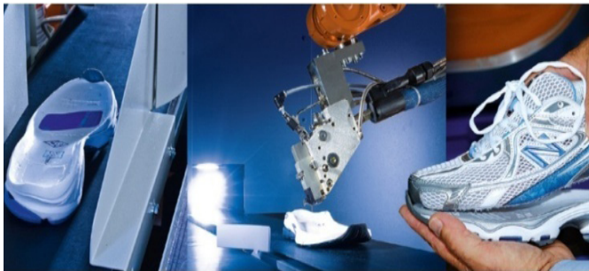
F.127 Automatic gluing
