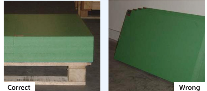
F.24 Correct (horizontal) and wrong storage (vertical) of cutting boards
