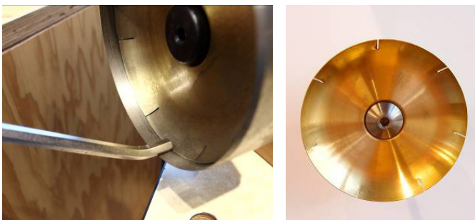
F.41 a - b Separators (important for proper dust exhausting and to protect the inside of the bell knife from skiving waste)
