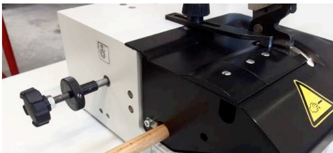
F.42 A holder keeps the dressing tool in its correct position and the edge of the grinding stone flat and not rounded. This guarantees efficient exhausting and proper grinding.
