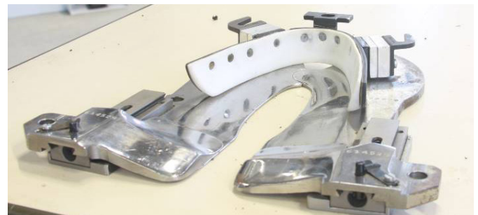
F.88 The Teflon band and the wipers are the most important tools for toe lasting
