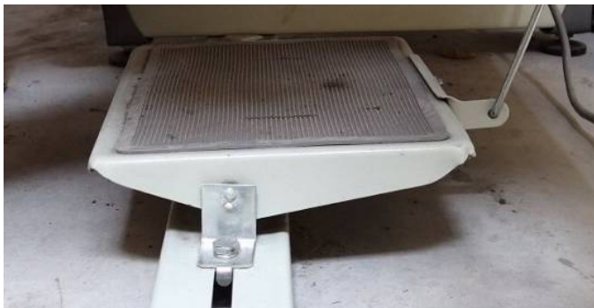
F.159 Wrong position of speed treadle
