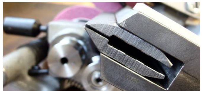
F.26 These clamps keep the upper and bottom position of the bell knife
