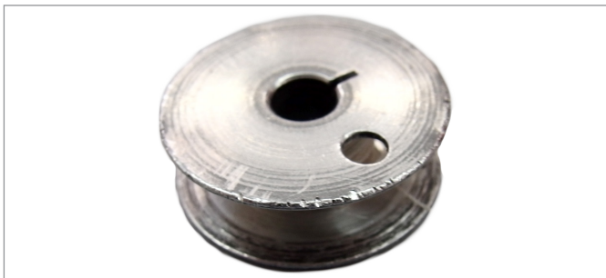
F.66 This is an example of an expensive computer-controlled stitching machine which was not operated with the original bobbin. In addition company did not want to spend 1€ for the correct screwdriver to change the needle so the workers used the cheap bobbin for changing the needle.
