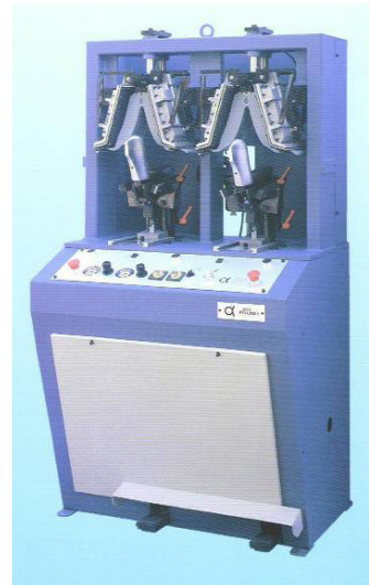
F.76 Basic backpart moulding machine for pre-moulded leather board counters with adhesive coating
