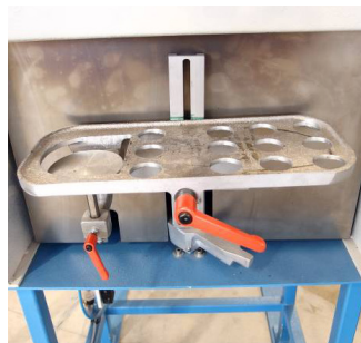
F.134 Adjustable height of sole support with separate adjustable heel support
