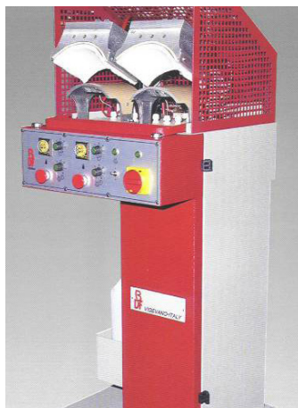
F.80 Classic clamp activation system (available as pair or half-pair version)
