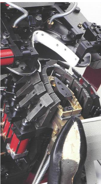
F.93 The hotmelt application crown requires relatively large amounts of energy to heat the hotmelt and the metal piece up to ~ 200 °C
