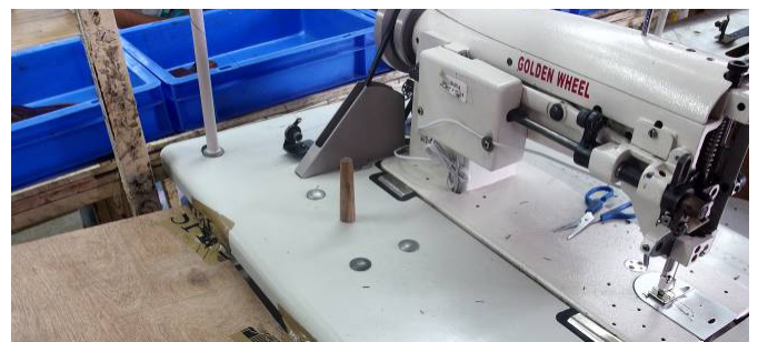
F.147 Some designs need a larger area to be placed on. This worktable extension (a simple board) is a cheap solution and saves a considerable amount of manipulation time
