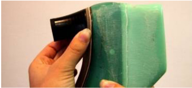
F.84 The bevelled insole must match the shape of the last bottom
