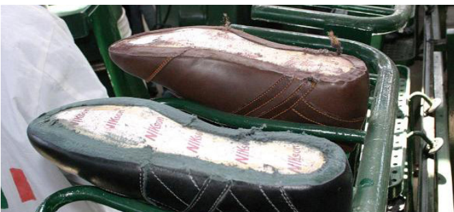
F.115 Another frequent mistake: When roughing dust remains on the surface, it will be covered with glue in the next step .... and will weaken the bonding strength.
