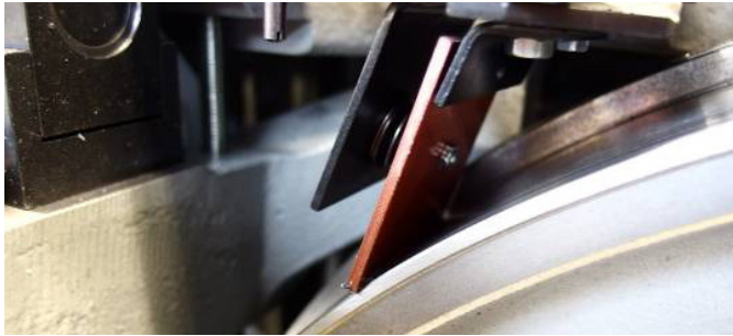
F.28 - Left Surface knife cleaning.
