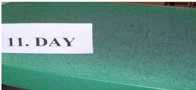
F.23 Wear of the cutting board after eleven working days (one day before planing scheduled for day 12). The shoe factory used only one side of the cutting board for the pictures. Cutting depth almost 2 cm.
