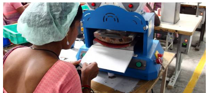
F.46 Toe puff ironing machine (work station can be organized both for standing or sitting)
