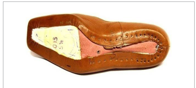
F.89 Perfectly lasted upper (no additional pressing or hammering)
