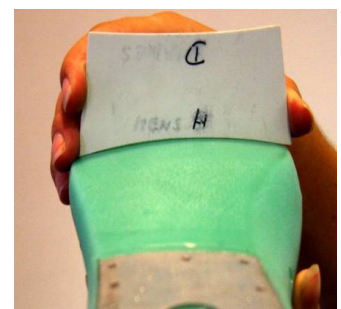
F.91 For a perfect lasting result, the bottom shape of the last and the shape of the wipers must match
