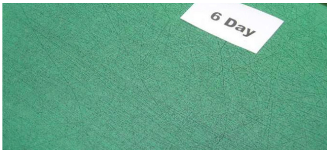
F.22 Wear of the cutting board after six working days: cutting depth 1.1 mm
