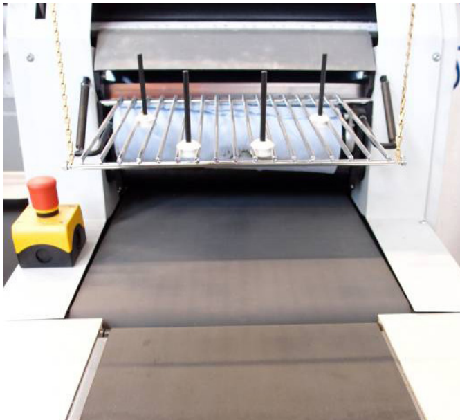
F.49 Conveyor-type ironing machine which can be operated by one worker. Insertion and output are on the same side. This machine is ideal for high-speed bulk production.
