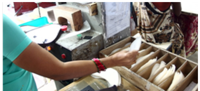
F.53 Example of a simple solution to organise toe puffs: Each size is stored in a dedicated compartment
