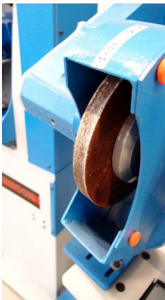
F.110 Example of a “vulcanised” wire brush
