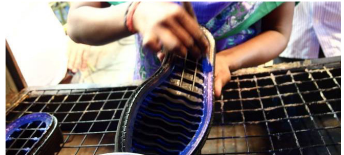
F.71 Example of a simple and efficient way to organise a gluing workplace
