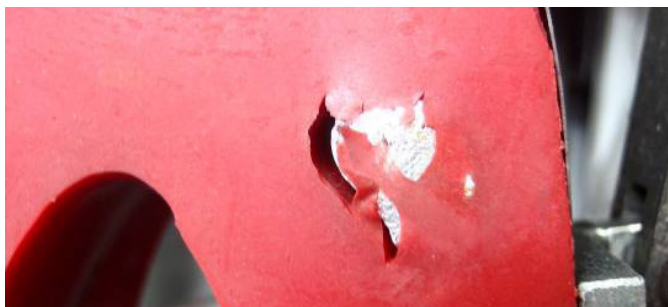
F.75 Accumulation of frequent mistakes: The heating bodies are not the original ones and the recommended working temperature was exceeded.
