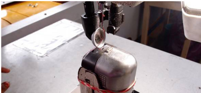
F.65 This is an example of what to avoid: Cheap thread, dirty machine, badly adjusted hook – in consequence, the stitching result will be poor and the thread risks breakage.
