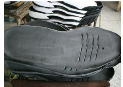
F.112 Roughing result of the widia tool
