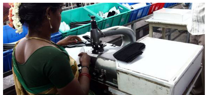
F.146 At this workplace, large skived pieces frequently fell down. A small box placed next to the machine solved the problem and increased quality and productivity
