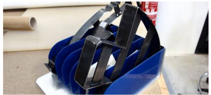
F.15 Correct storage of cutting dies is important
