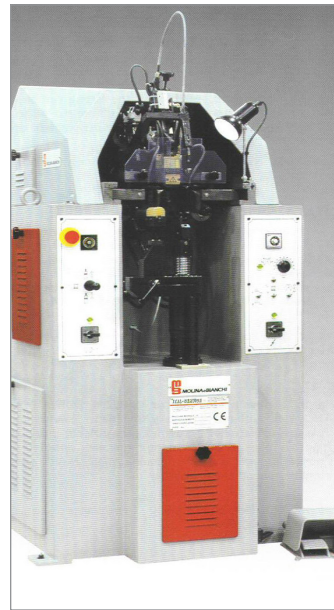
F.103 Seat lasting machine (with hotmelt or with “cold” cements applied by hand)
