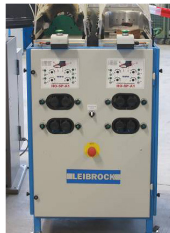
F.82 Activation system using overheated steam featuring the possibility to set different temperatures for different zones of the upper
