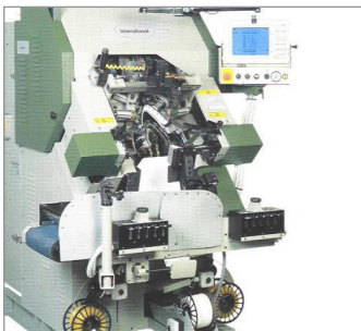
F.99 Fully electronic toe lasting machine with step motors
