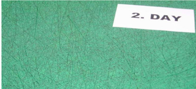
F.20 Wear of the cutting board after two working days: cutting depth 0.5 mm
