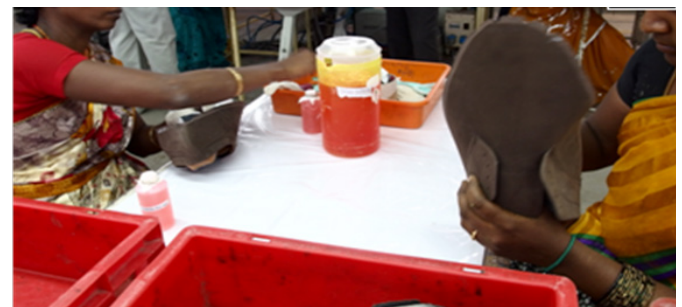
F.148 In this production, precise glue application by brush was problematic. A small bottle equipped with a textile tip and a larger can with a glue supply for 2 to 3 hours permits exact glue application and reduces the solvent evaporation in the working area.
