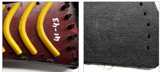
F.16 / F.17 Cutting dies can be equipped with punchers, prickers, or markers, which can make subsequent work steps redundant
