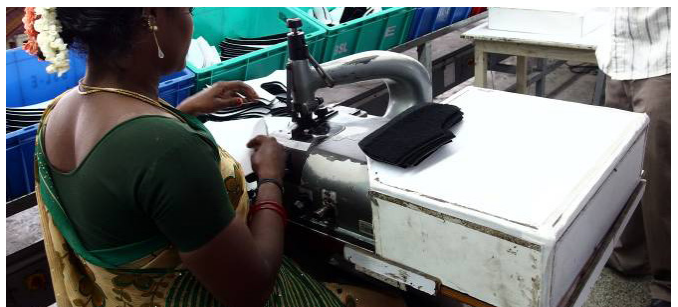
F.54 Example of a skiving workplace: The skived parts can easily be put down without risking to fall down
