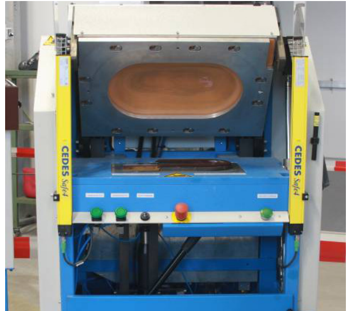
F.140 Double membrane pneumatic sole press with sole activation machine
