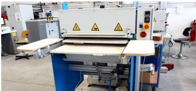
F.48 Ironing machine with moving shelves
