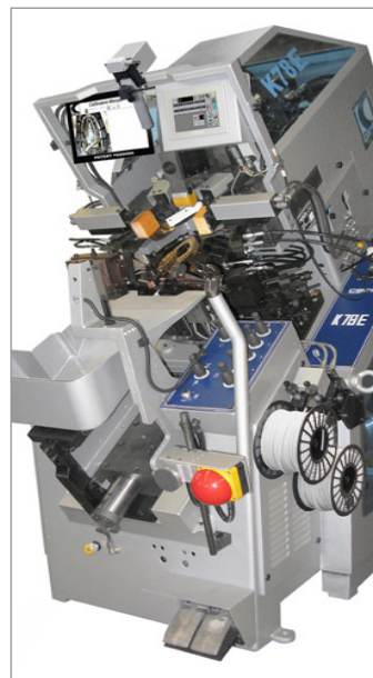
F.96 Toe lasting machine equipped with a camera and an additional screen. The first lasted shoe from each pair is photographed and the picture is displayed on the screen. At the moment of elongation of the second shoe, both vamp shapes appear on the screen. This system helps to produce identical lasting results for left and right shoes while keeping fast cycle times and simultaneously avoiding reworks and rejects.
