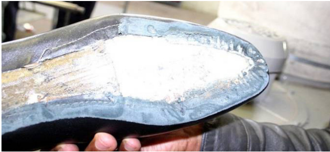
F.114 Example of an overroughed upper: the white interlining is shining through. The strength of the sole bond will now completely depend on the structure strength of the lining and interlining.
