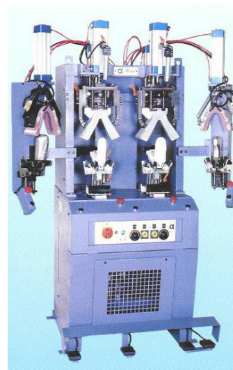
F.77 Hot and cold backpart moulding machine
