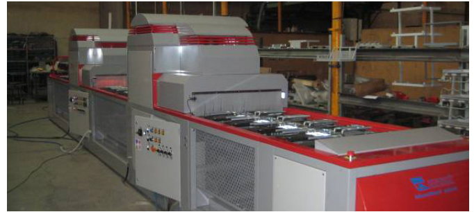
F.132 Drying line with vacuum dryers
