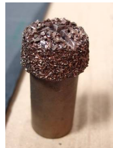
F.111 Special widia tool for 3D sole
