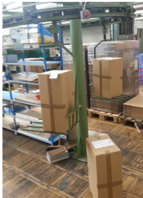
F7. Free hanging conveyor for box transport from production to warehouse
