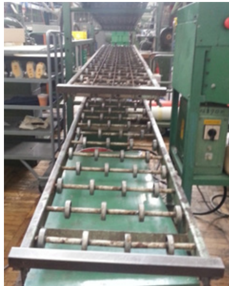
F6. Roller conveyor for short transport between two working phases
