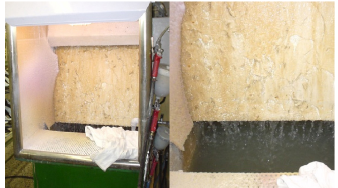
F.7 Water-curtain finishing booths
